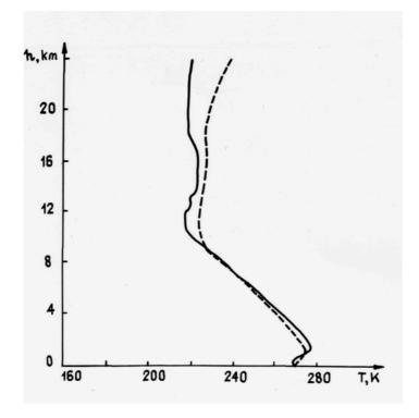
Fig.1. Restoration of the temperature profile with a strong inversion in the boundary layer by the method of statistical regularization for  $\delta \varepsilon = 10$ ". A solid line is the initial profile, a dotted line is the retrieved one.
