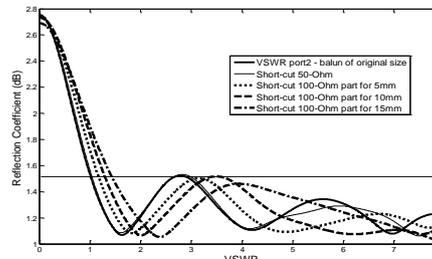
**Fig. 3.** Simulated results. a)-transmission coefficient obtained for transformers with different length of CPS; b)- VSWR for port 2 of balun with different length of CPS.
