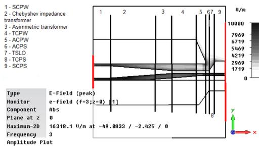
**Fig.1.** Layout CPW to CPS transformer. Physical configuration with simulation results for the electric field amplitude and equivalent-circuits model.
