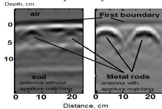
**Fig. 5.** Experimental results for antennas without (left) and with (right) aperture matching.
