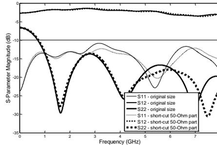
**Fig.2.** Simulated S-parameters of the transformer.
