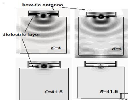
**Fig. 4.** Simulation results. Electric field amplitude for the bow-tie dipoles with (left) and without (right) the dielectric layer in the aperture at frequency of 2 GHz.
