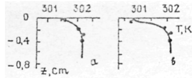
Fig.2. Retrieval of natural thermal film in water. Points - contact measurements, solid line - retrieval. a - without wind, b- in presence of wind
